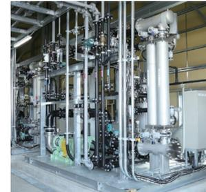
This technology uses ceramic membranes to treat produced water, by removing oil and suspended solids. Ceramic membranes have higher resistance to chemical and oil fouling and have a larger filtration contact area, which leads to less elements and/or units being required to deliver equivalent treatment capacities.
