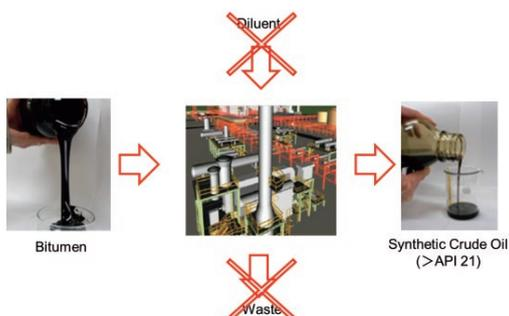
SCWC is a technology for upgrading high viscosity, extra heavy oils (e.g. oilsands) into synthetic crude for pipeline transportation. This process does not emit any waste, making it an environment-friendly technology.
